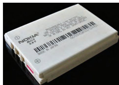
Fig 4.10 Lithium Ion Battery
