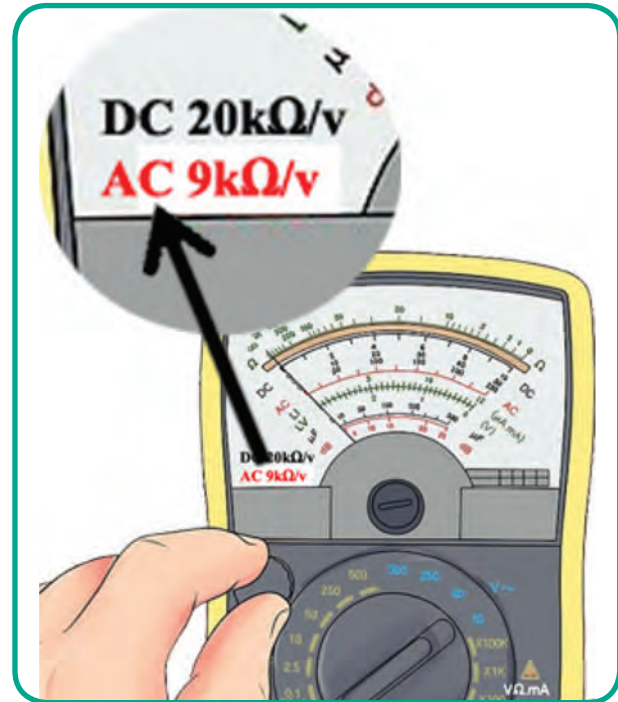
Figure 10.9 Sensitivity of an analog multimeter
