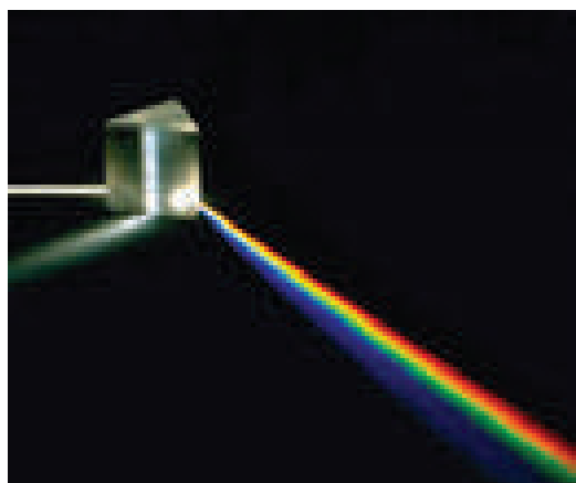
Figure 5.12 White light passed through prism – dispersion
