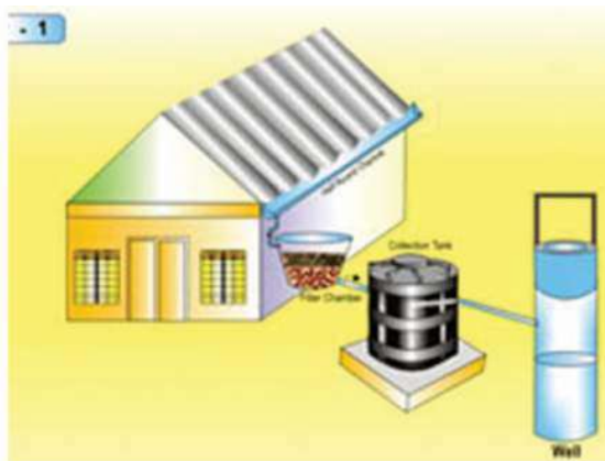
Rain water into wells
