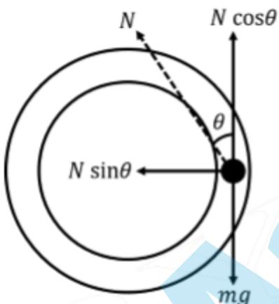
The components of Normal reaction for cyclist need to satisfy the equation of dynamics i.e. supporting the weight & centripetal force.
