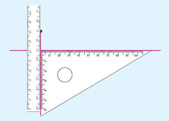
Now by shifting the set square upward and putting its square corner at the point, we can draw the parallel:
