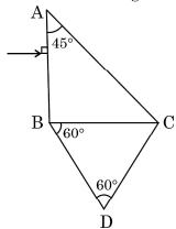
The critical angles for the two prisms with respect to air are 41.1° and 45° respectively. Trace the path of the ray through the combination.
