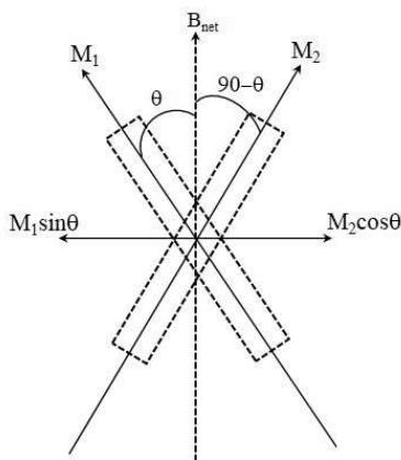
Components of  $M_1$  and  $M_2$ , in the direction perpendicular to magnetic meridian, must be cancelled.
