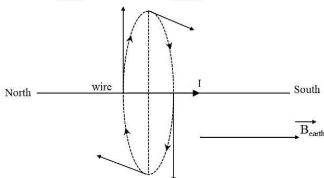
The magnetic field line around the straight wire is shown above. The direction of magnetic field at a point, will be along the tangent drawn to the field line, at that point.
