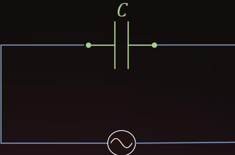
$$\begin{aligned} \varepsilon &= \varepsilon_0 \sin \omega t \\ i &= i_0 \sin \left( \omega t + \frac{\pi}{2} \right) \end{aligned}$$
