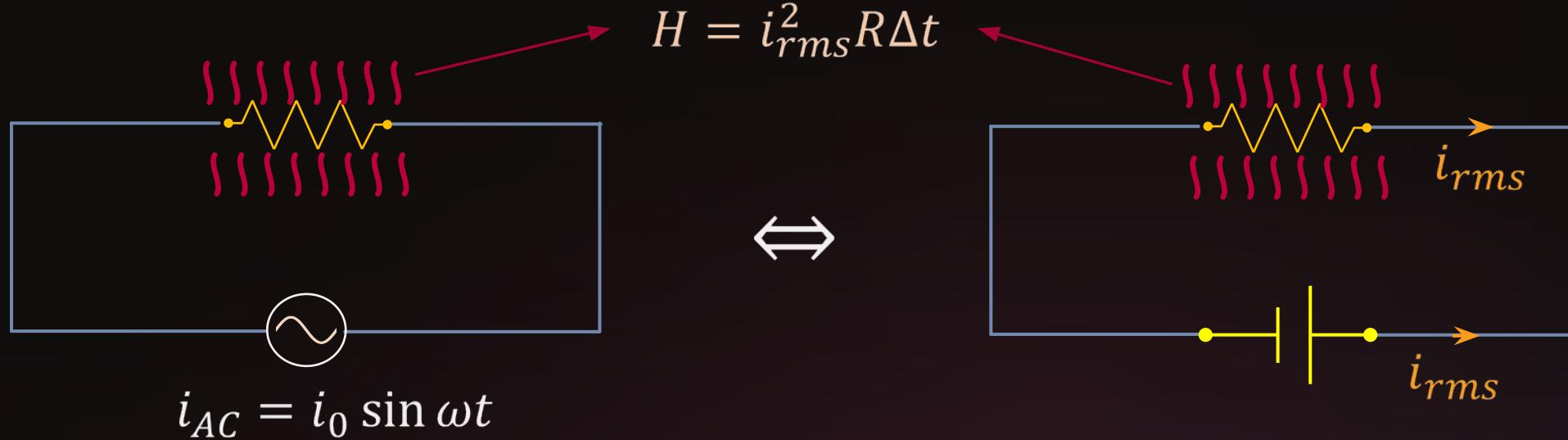
RMS value of a given AC can be defined as that DC value which produces same heat in a resistance which the AC produces in that resistance in same duration.
