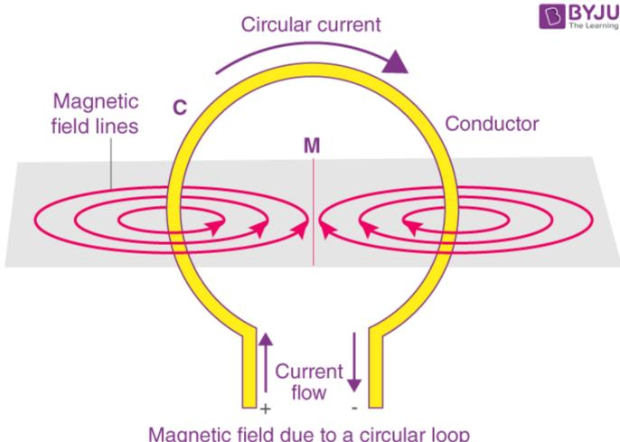
Magnetic field due to a circular loop
