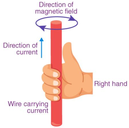
Consider a straight current-carrying wire which is held vertically in the upward direction from A to B. The wire is held as in the given figure to find the direction of the magnetic field lines that is produced when the current flows through the wire. The thumb gives the direction of the current. The fingers that are encircled around the wire gives the direction of the magnetic field lines. The direction of the magnetic field lines is in the anticlockwise direction.
