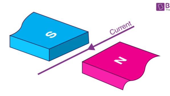
The force on the wire due to the magnet is directed:
