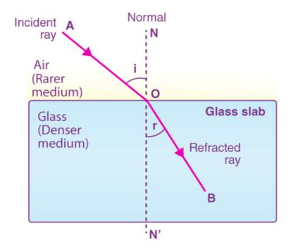
Q27. When a light ray passes from air into glass, what happens to its speed? Draw a diagram to show which way the ray of light bends.
