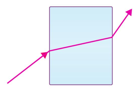
Q24. What is meant by the angle of incidence and the angle of refraction for a ray of light? Draw a labelled ray diagram to show the angle of incidence and the angle of refraction for a refracted ray of light.
