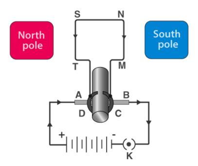
When current is made to flow through the coil MNST by closing the switch, the coil starts to rotate in the anticlockwise direction. This is due to the downward force acting on the length MN and simultaneously an upward force acting along the length ST. As a result of which, the coil rotates in the anticlockwise direction. Current in the length MN flows from
