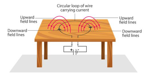
For the downward direction of the current, the direction of the magnetic field will be as if emerging from the table outside the loop and merging with the table inside the loop. Similarly, for current flowing in an upward direction, the direction of the magnetic field will be as if they are emerging from the table outside the loop and merging with the table inside the loop, as shown in the figure.
