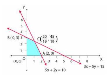
O (0,0), A (2,0), B (0,3) and C (20/19,45/19) are the corner points of the feasible region. The values of Z at these corner points are given below.
