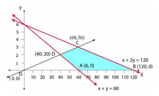
A (60, 0), B (120, 0), C (60, 30), and D (40, 20) are the corner points of the feasible region. The values of Z at these corner points are given below.
