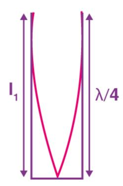
This kind of system creates odd harmonics. We know that the fundamental note in a closed pipe is written as:
