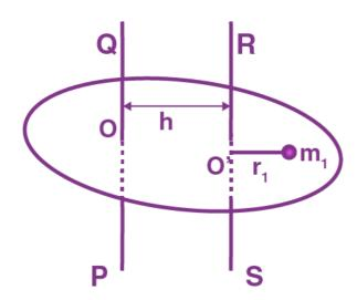
Suppose a rigid body is made up of n number of particles, having masses  $m_1, m_2, m_3, \ldots, m_n$ , at perpendicular distances  $r_1, r_2, r_3, \ldots, r_n$  respectively from the centre of mass C of the rigid body.
