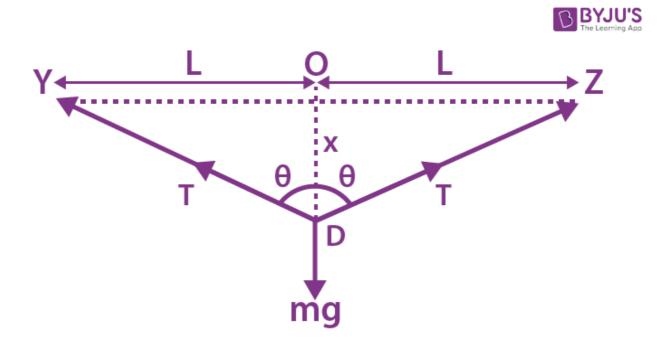
Let YZ be the mild steel wire of length 2l = 2m and cross-sectional area  $A = 0.60 \times 10^{-2} \text{ cm}^2$ . Let the mass of m = 100 g = 0.1 kg be hung from the midpoint O, as shown in the figure. And let x be the depression at the midpoint, i.e., OD
