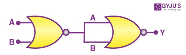
(Hint: A = 0, B = 1, then A and B inputs of the second NOR gate will be 0 and hence, Y=1. Similarly, work out the values of Y for other combinations of A and B. Compare with the truth table of OR, AND, NOT gates and find the correct one.)
