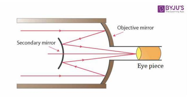
The distance between the objective mirror and the secondary mirror, d = 20 mm
