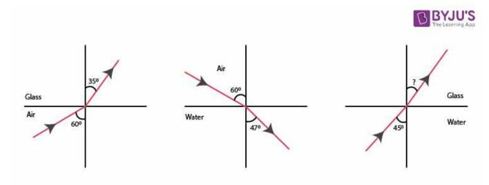
The figures above show the refraction of a ray in air incident at 60° with the normal to a glass-air and water-air interface, respectively. Predict the angle of refraction in a glass when the angle of incidence in water is 45° with the normal to a water-glass interface.
