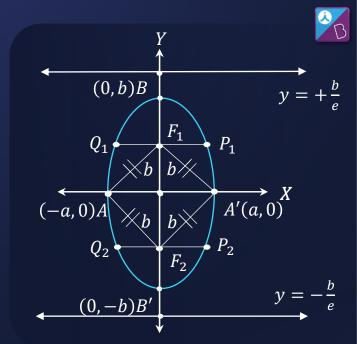
The ellipse is symmetric about both X and Y-axis.
