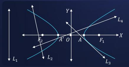
A line can intersect Hyperbola at not more than 2 points as when we solve equation of line (linear) with the equation of hyperbola (2<sup>nd</sup> degree), we get a Quadratic Equation, which has at most 2 distinct real roots.
