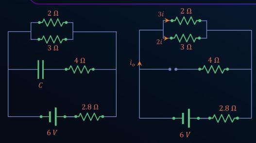
At steady state, current across the condenser is zero and behaves as an open circuit (branch)
