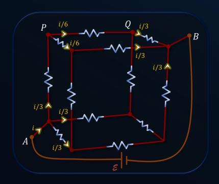
Applying KVL in the loop APQBA on starting from point P, we get,
