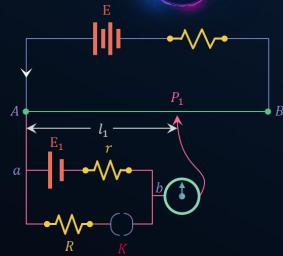
• When the key is open, no current flows through the secondary circuit. If the null point is found at point P (length  $l_1$ ), then,
