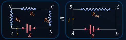
$$R_{eq} = R_1 + R_2 + R_3$$
