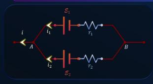
Net resistance,  $\frac{1}{r_{eq}} = \frac{1}{r_1} + \frac{1}{r_2}$
