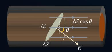
• If the current  $\Delta i$  exists through an area  $\Delta S$  which makes an angle  $\theta$  with the current, as shown in the figure, then
