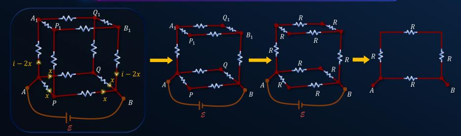
The circuit has input & output symmetry & junction P & Q are redundant. Therefore current through branches  $PP_1$  &  $QQ_1$  are zero.
