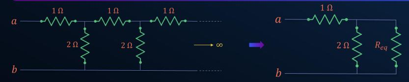
• Equivalent resistance between a and b is,
