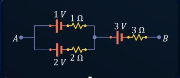
$$A \bullet \qquad \begin{array}{c} \frac{4}{3} V \quad \frac{2}{3} \Omega \\ E' \quad r' \end{array}$$
