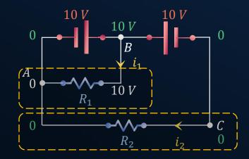
• Current through resistor  $R_1 \& R_2$ .
