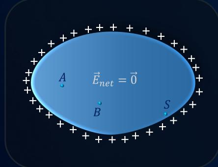
Net electric field inside a conductor is zero.
