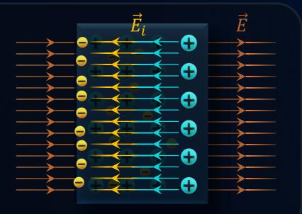
When an isolated conductor is placed in an external electric field, internal division of charges occurs, resulting an internal Electric Field ( $\vec{E}_i$ ) in the direction opposite to external Field ( $\vec{E}$ ). This phenomenon is call Polarisation of charges.
