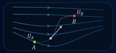
The change in electric potential is defined as the change in potential energy per unit charge.
