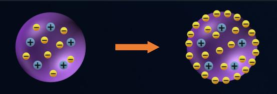
Excess charge given to an isolated conductor redistributes itself on the conductor's surface in order to minimize the potential energy and maximize stability.
