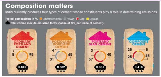
Figure: Types of cement produced in India Source: Down to Earth
