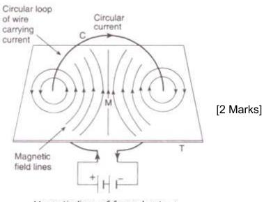
Magnetic lines of force due to a circular wire carrying current
