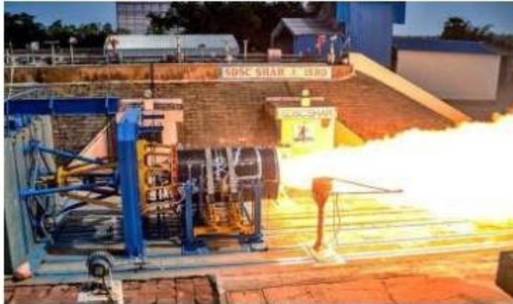
Kalam-250, the second stage of Vikram-1 launch vehicle, being test fired by Skyroot Aerospace at Sriharikota in A.P. on Wednesday.
